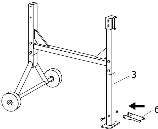
Install the pedal, pos. 6 on the support, pos. 3, fix it with the bolt M8 x 70 and the nut M8 with a stopper ring.
