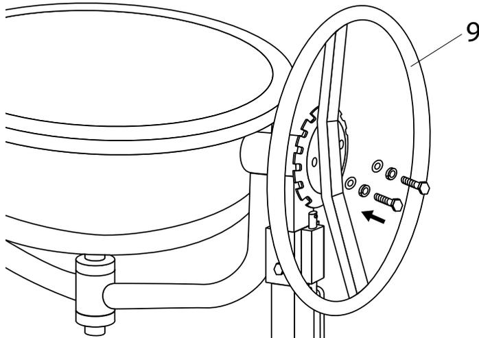
Install the steering wheel, pos. 9, fix it with bolts M8 x 16 with lock washers, pos. 8 and the washer, pos.
