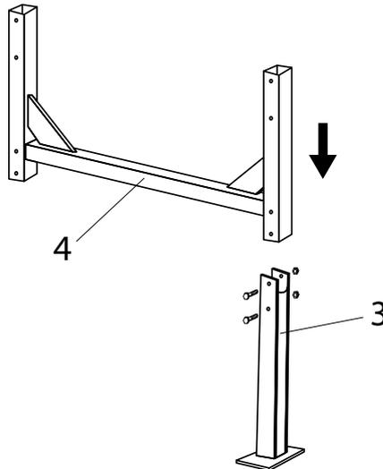
Connect the support, pos. 3 with the frame, pos. 4 by means of bolts M8 x 65 and fix with M8 nuts. The support should be installed from the frame side with 3 openings (for the CM120 model - from the spring side).
