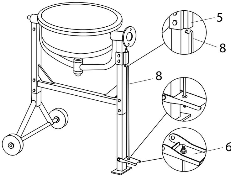
Install the washer, pos. 6 on the pull rod, pos. 8, and attach it to the pedal, pos. 6. Install the washer 5 and secure the pull rod with two nuts M5, as shown in the figure. Attach for the pull rod to the rod of the fixing block 5.
