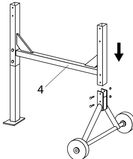
Connect the wheel support complete with the frame, pos. 4 by means of bolts M8 x 65 and fix with M8 nuts.
