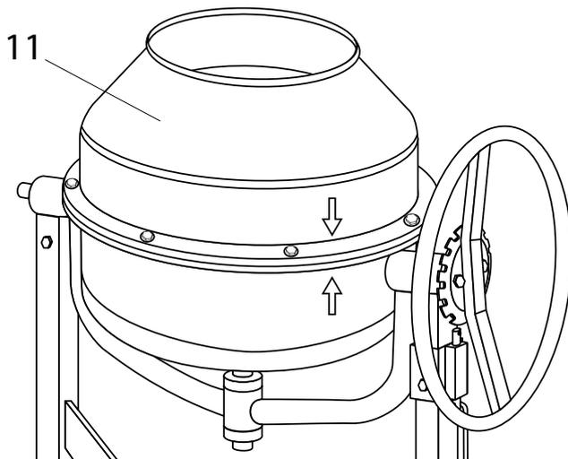
Install the upper drum, pos. 11 on the lower one according to the stamped arrows, tighten the bolts.
