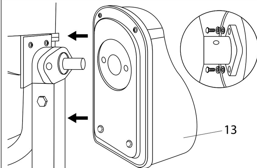
Connect the drive, pos.13 and fix it with bolts M8 x25, lock washer, pos. 8 and washer, pos. 8.
