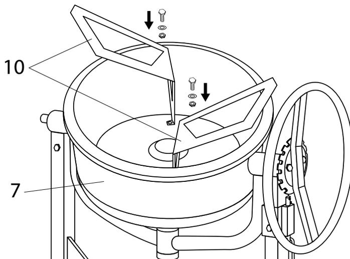
Install blades for mixing of pos. 10 in the lower drum of pos. 7 to fix by bolts of M8x16, washers 8 and nuts of M8.
