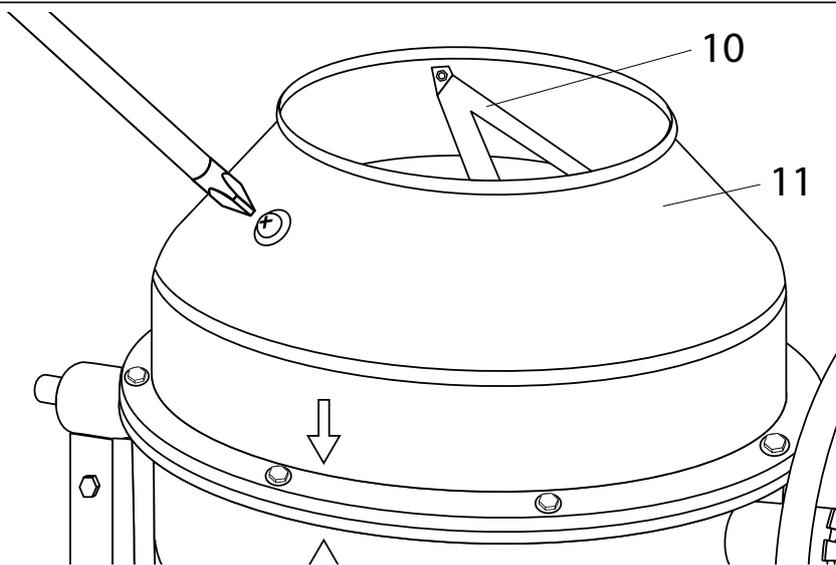
Fix an upper part of blades, pos. 10 on an upper drum, pos. 11 with the screws M8 x16, washers, pos. 8, nuts m8.
