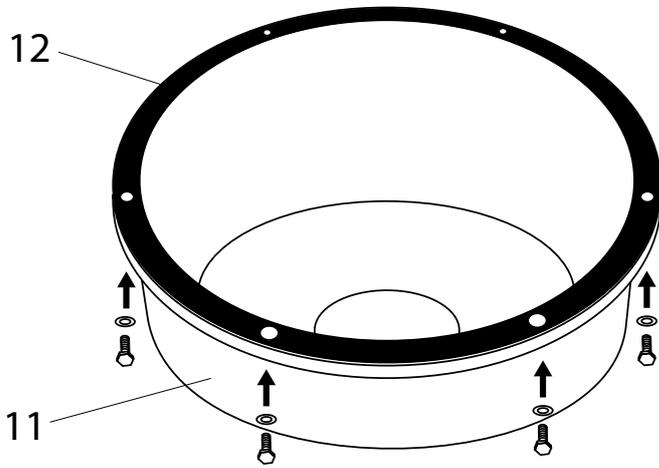
Install 6 sets of M6 x16 screws and washers, pos. 6 in the openings of an upper drum, pos. 11, install the seal, pos. 12, as shown in the figure.
